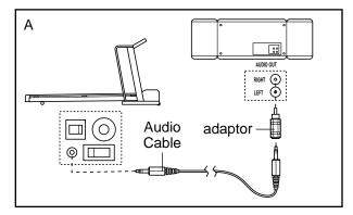
other end of the cable into the included adaptor. Plug the adaptor into an AUDIO OUT jack on your stereo.
